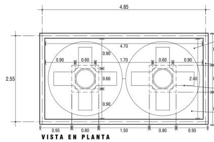
LOSA DE CONCRETO DE 12 cms. DE ESPESOR, DE  $f_c=250$  Kg/cm<sup>2</sup>, ARMADA CON VARILLA DE  $\frac{3}{4}$ " @ 30 cms.
